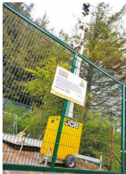
Temporary/mobile alarm/CCTV unit
